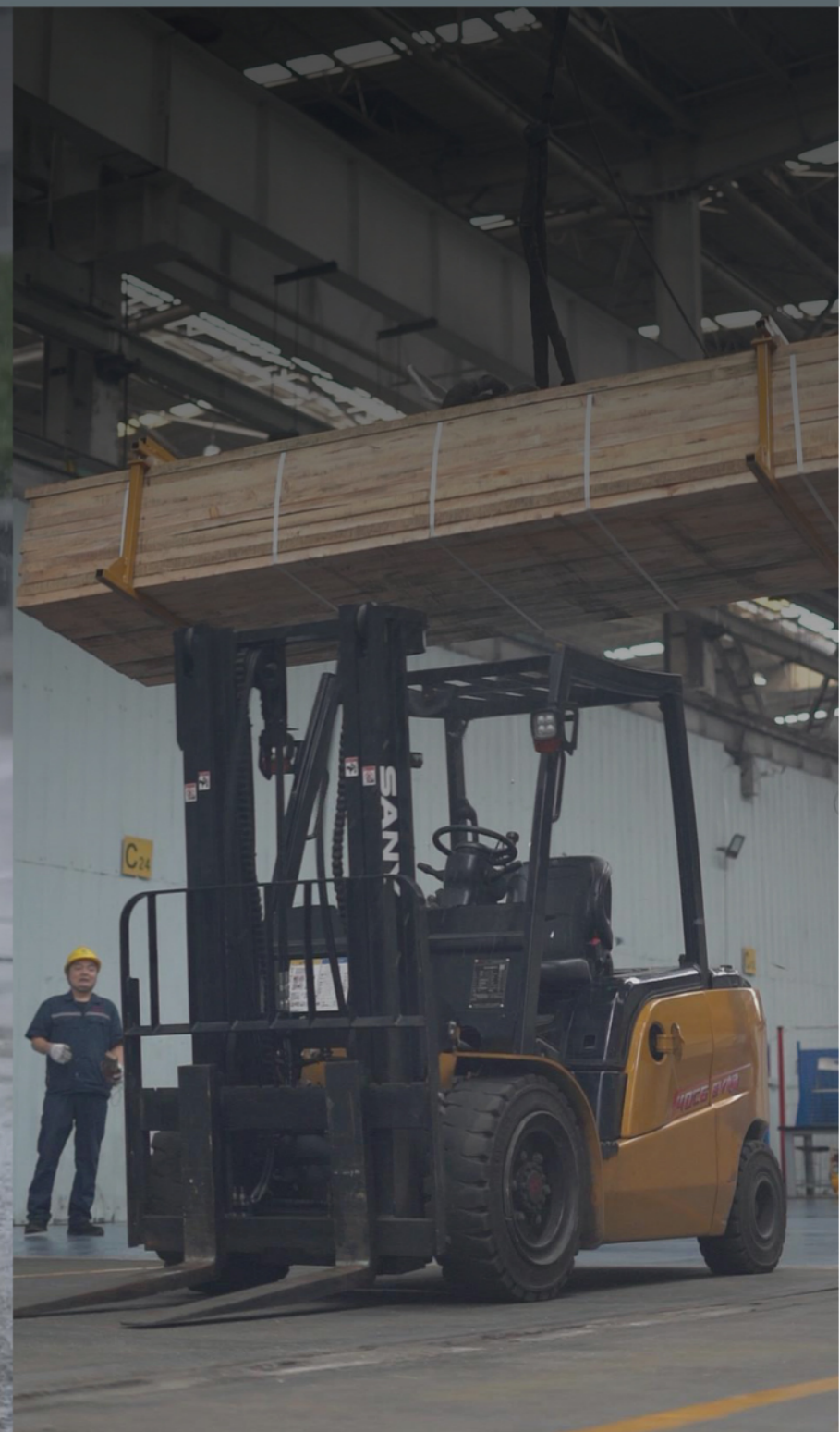
Full marks passed the protective roof frame impact test
