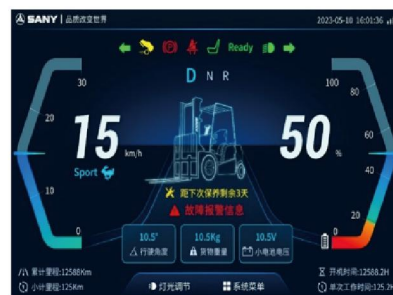
标配智能仪表7寸大屏， 触摸操控，方便快捷 Standard intelligent instrument with 7-inch large screen, for intuitive and easy operation
