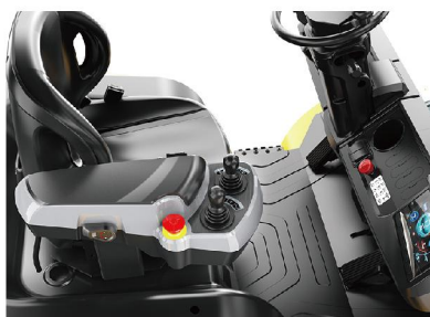
减震座椅，无惧颠簸，消除疲劳 座椅标配OPS开关，离位感应 Shock-absorbing seats to eliminate fatigue, equipped with OPS switch and seat occupancy sensor
