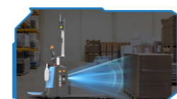
Standard pallet adaptive identification 3D LiDAR sensing
